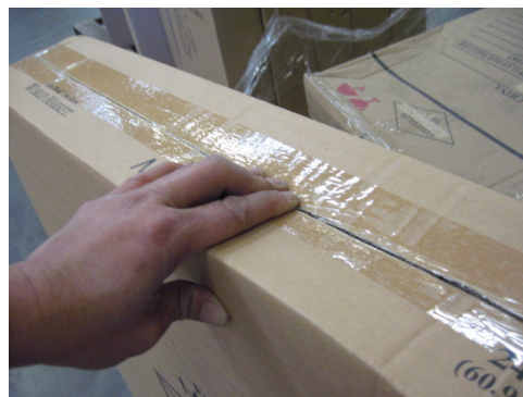
Figure 9: Example of the weak point of an RSC seam
