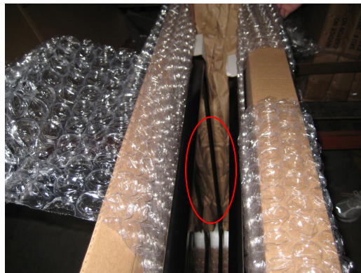
Figure 5: A sufficient amount of packaging material must be placed in between frames to prevent glass surfaces from contact upon impact during transit.
